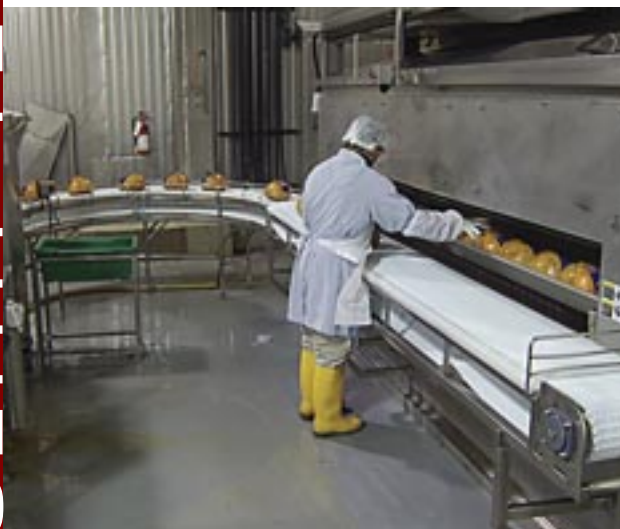
This process heats the external face of the sealed-in-bag fully cooked turkey breast to eliminate potential microbiological issues.
